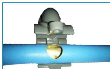
Step 5: Aligning the Droplet to the hole
